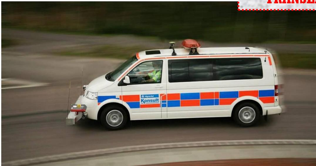
This study shows that enhanced marking on road maintenance vehicles led to the increased attention of road users, resulting in slower speeds. SRA orange/blue Battenburg patterns reduced their speed by 3 km / h in the medium, and the percentage of vehicles that were more than 15 km/h over the speed limit fell by 90%. *Attentive driving prevents the "foolish accident."*
