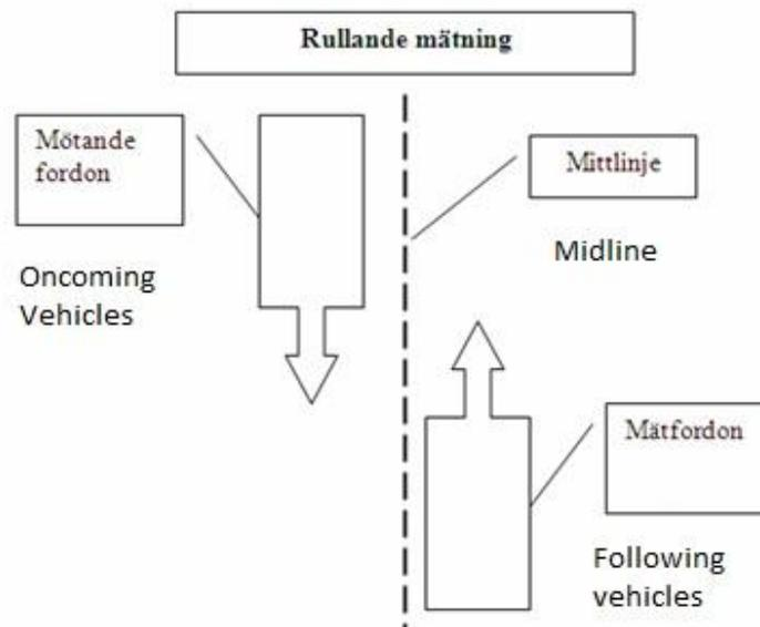
Figure 10. Vehicle Location at the center line of measurement (rolling survey vehicles / radar)
