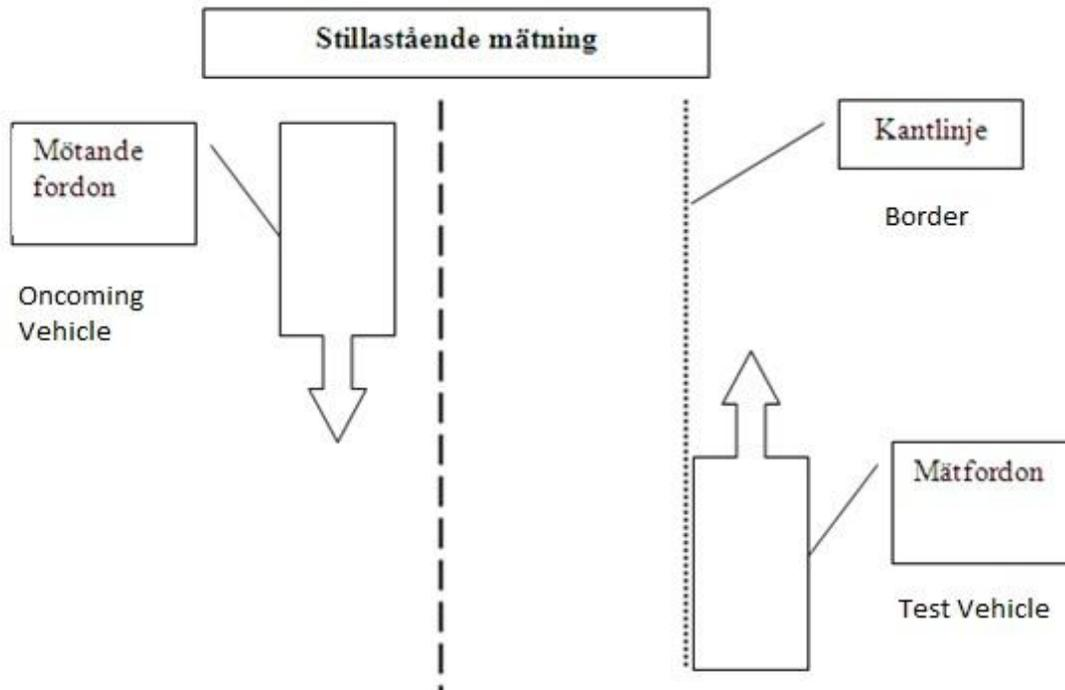
Figure 8 Vehicle location at *inspection stop* (stationary measuring car/radar)
